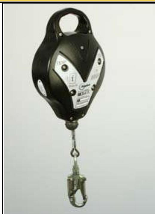
A lighter weight and smaller block than the RGA2, the RGA26 is also a multi purpose fall arrest block, which allows uninhibited movement during normal working activity. The carrying handle is part of the cast alloy housing and can be connected to the anchorage point using soft slings or a karabiner.
