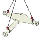
Comment: Rate as indicated only in cases where the load appears to be reasonably equally distributed between all three legs. If two are obviously supporting most of the load, rate at 2/3 of the marked working load.
