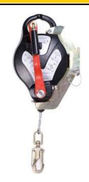
The RGA4 is a three way retrieval block fitted with an up/down winch mechanism and the standard fall arrest capability. This unit can be used as a standard fall arrest block, but in the event of a fall, the operative can be winched up or down to safety almost immediately. As most rescue systems lower the casualty, the RGA4 can raise the operative to safe area, if the area below is unsuitable.
