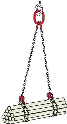
**WLL:** The WLL should be no more than 80% of the WLL for a two leg reeved sling.
